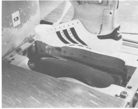
FIG. 2—In direct attach method, the lasted shoe upper is lowered into the mold assembly, which then closes tightly around it, allowing injection of outsole material directly onto shoe upper.
