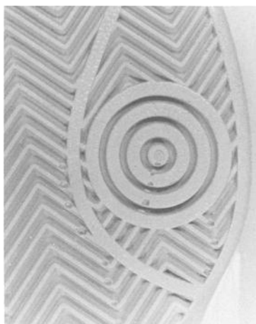
FIG. 11—Most air bubbles favor valleys of this herringbone pattern and bottom of circle pattern because direction of expansion is from toe to heel.
