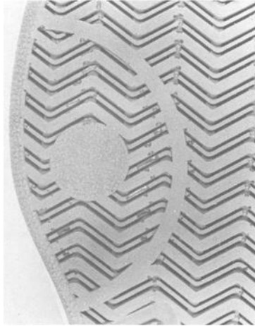
FIG. 1—Polyurethane outsole showing air bubbles on surface.
