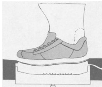
FIG. 3—Shoe upper, on a last, being lowered into mold assembly in a one-step direct attach operation.
